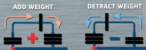
THE UNIQUE PATENTED VARIABLE LOADING SYSTEM. THE LOAD IS EASILY CHANGE BY MOVING THE WEIGHTS ALONG THE RAILS
