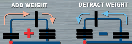
THE UNIQUE PATENTED VARIABLE LOADING SYSTEM. THE LOAD IS EASILY CHANGE BY MOVING THE WEIGHTS ALONG THE RAILS
